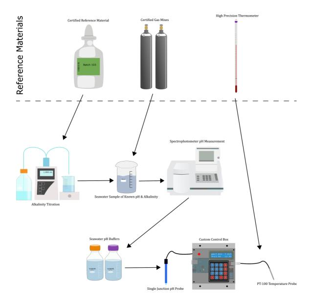
Figure 2. Flow chart of calibration protocol used in this study.
